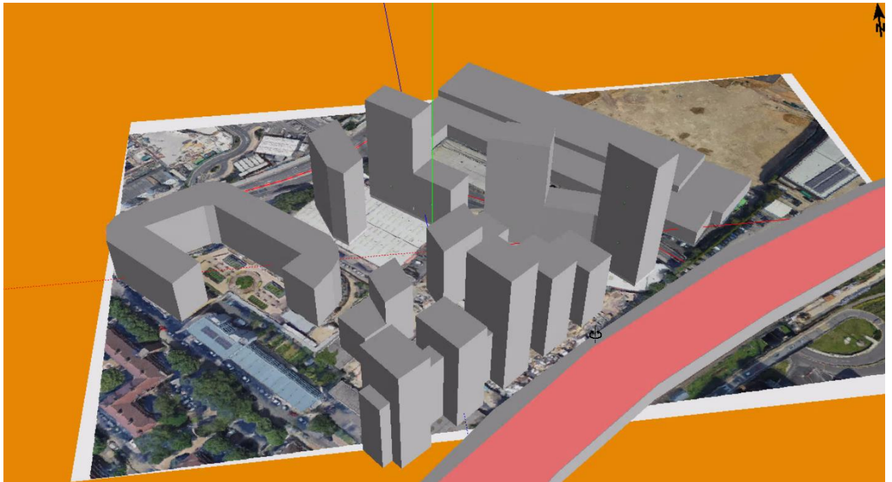
Figure 4. SoundPLAN noise model with the proposed buildings
