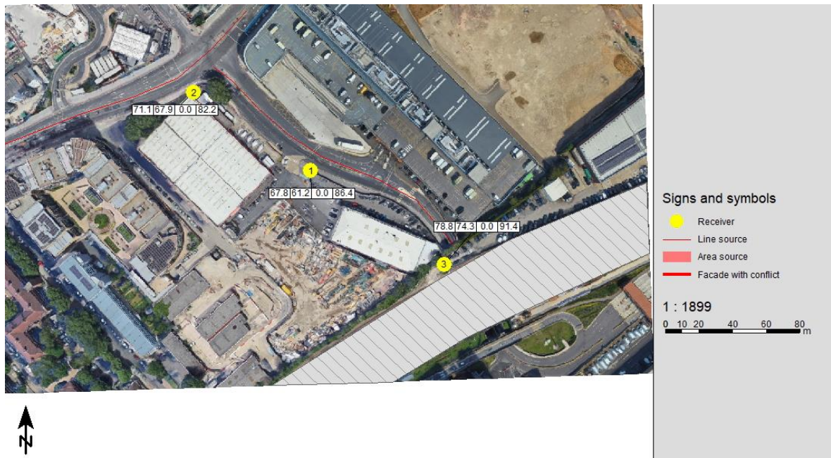
Figure 3. SoundPlan noise model calibration map
