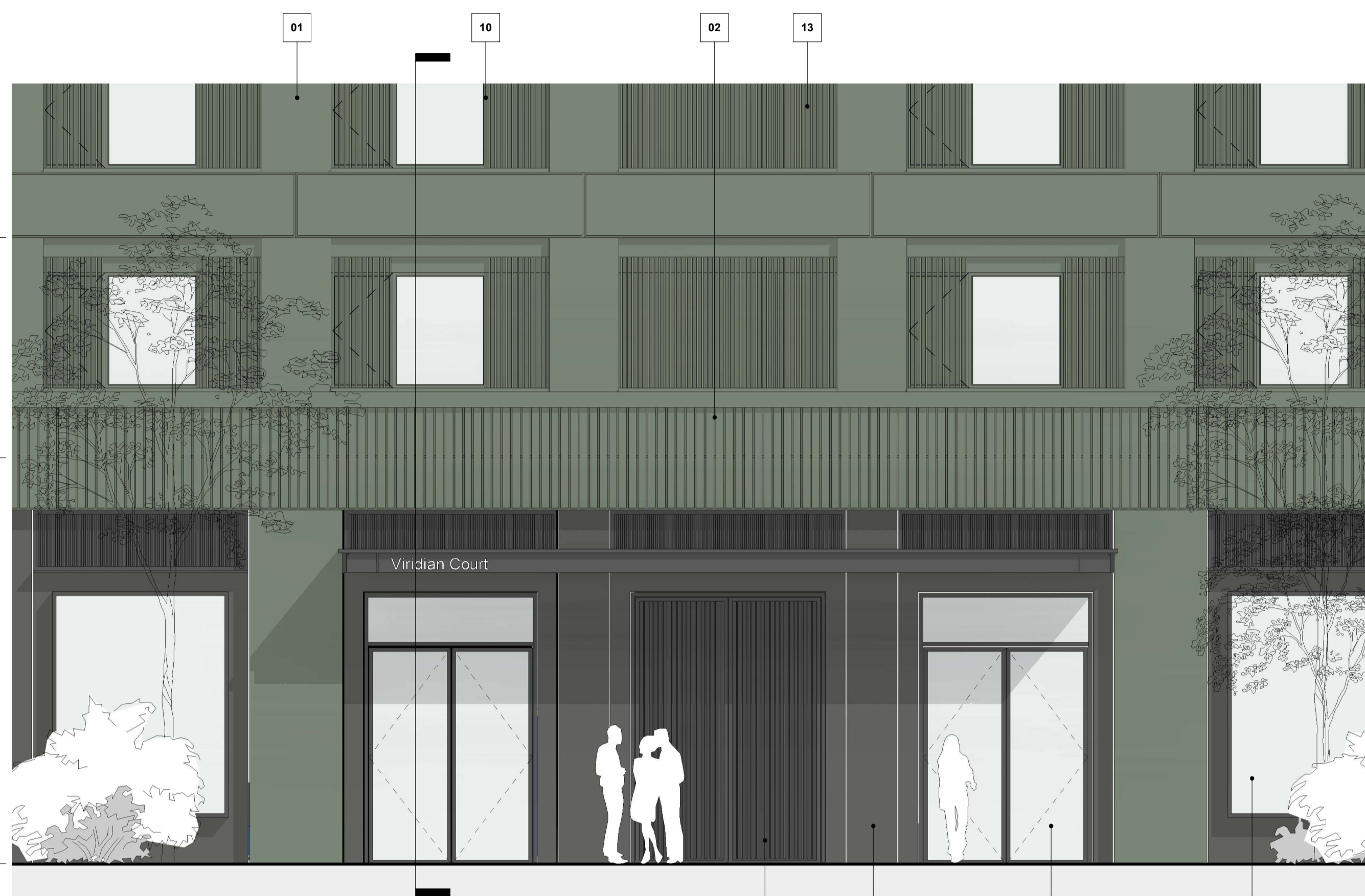
Bay Study Plot 02 - South West Entrance Elevation 1 : 50
