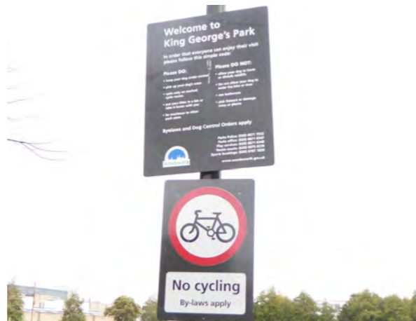
Signage is at high level and non-accessible
