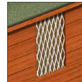
Internal diamond mesh grille over shed window
