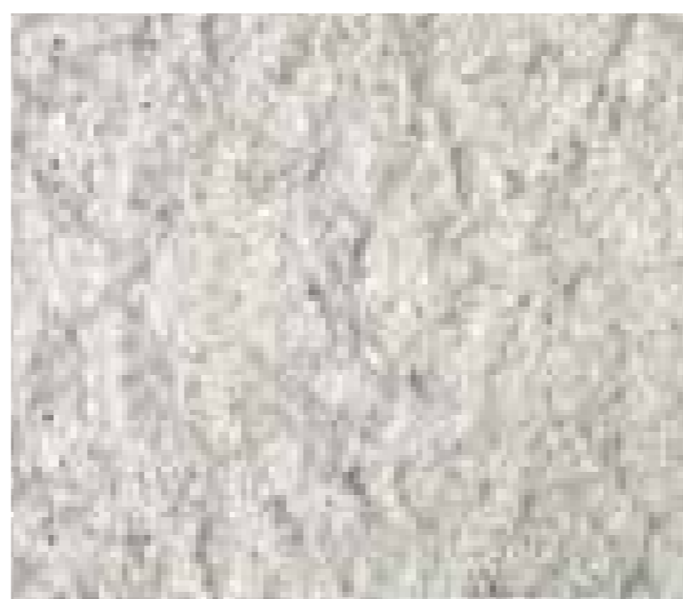
Grit blasted, form-lined precast concrete
