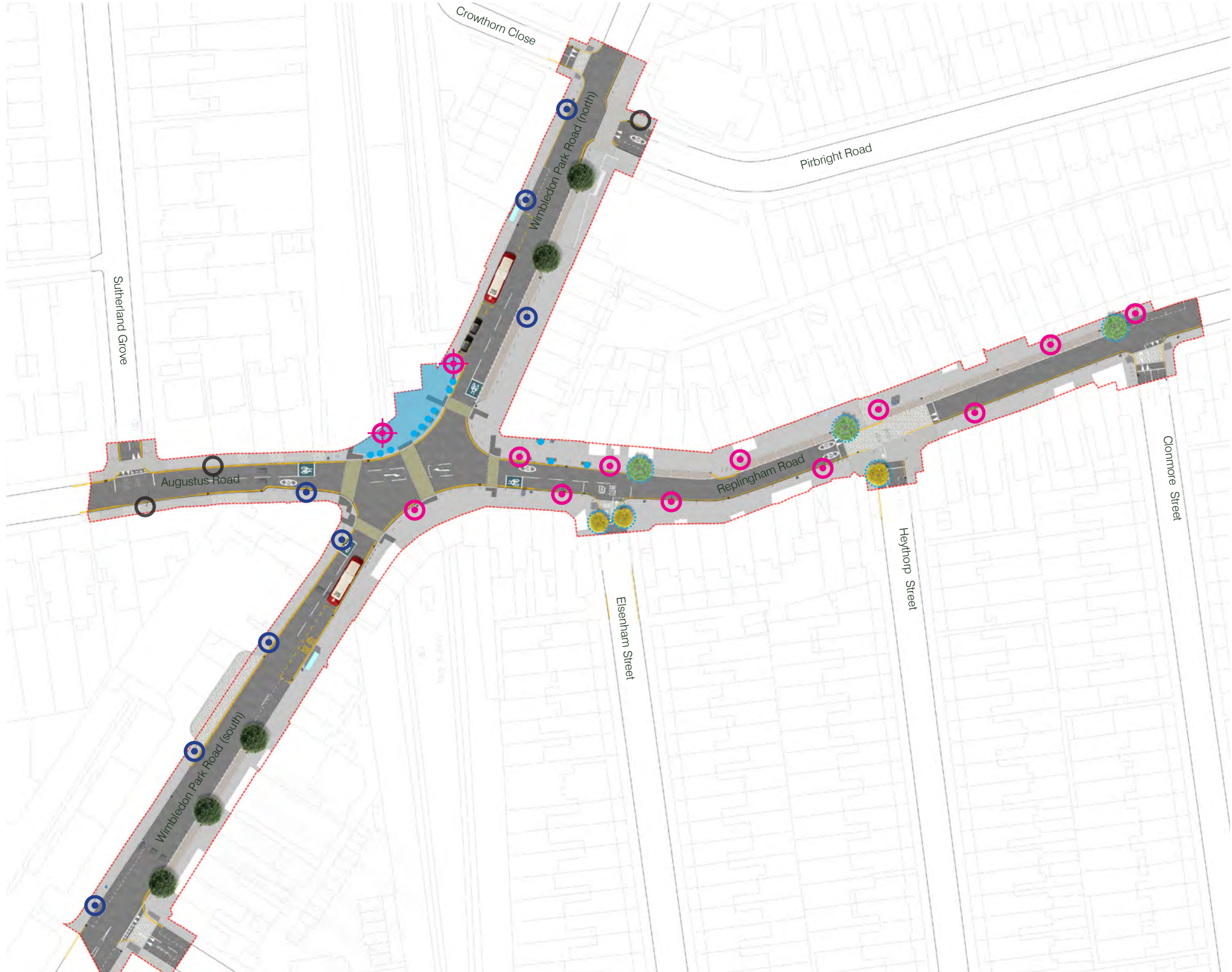
Figure 28. Plan showing street and feature lighting locations
