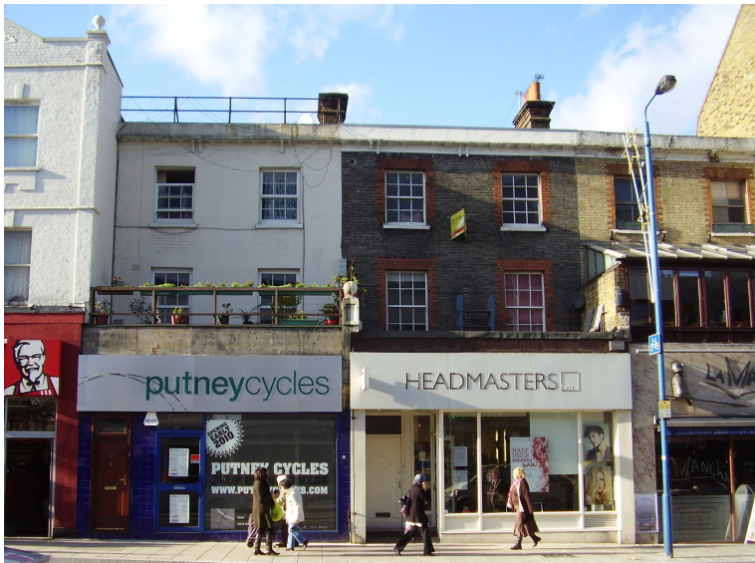
Figure 24 : Nos. 32-36 Putney High Street. The unpainted brick and six-over-six paned sashes would have been features of the whole group when first built
