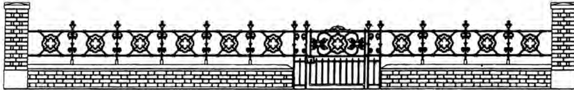
Figure 68 : Cast iron components making up a typical front boundary treatment with gate. (Note the absence of brick piers either side of the gate)
