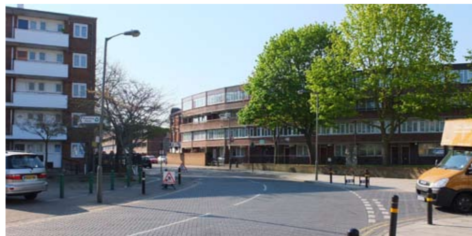
Raised tables reduce traffic speeds at junctions and can use attractive materials
