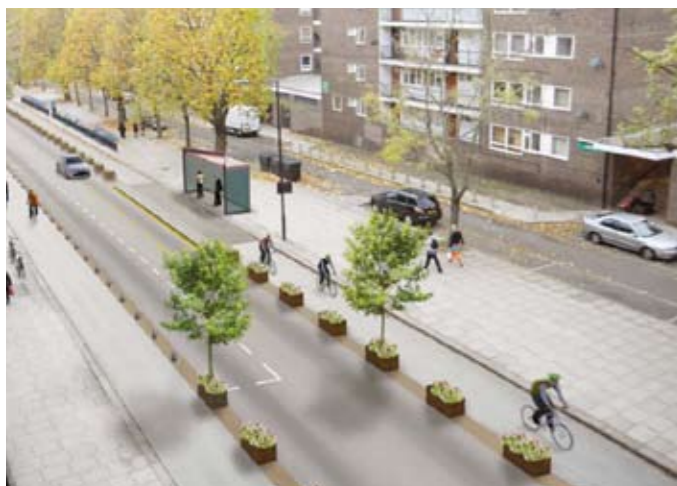
Planters and rubber studs are used to provide light segregation
