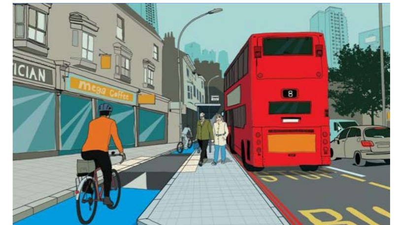
Floating bus stops reduce conflict between cyclists, buses and motor vehicles, improve traffic flow and support continuous routes
