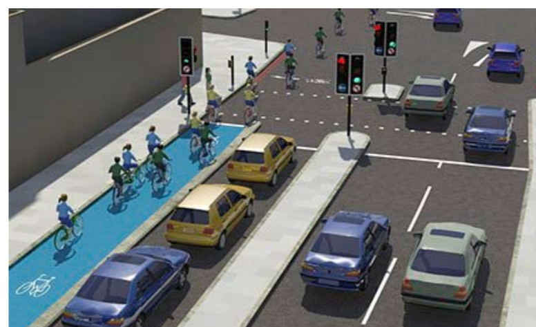
Junctions separate bicycle and motor traffic in space and time
