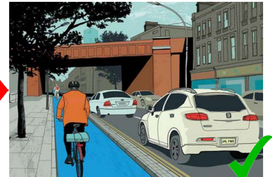
Existing inconsistent cycle lanes replaced by continuous segregated tracks
