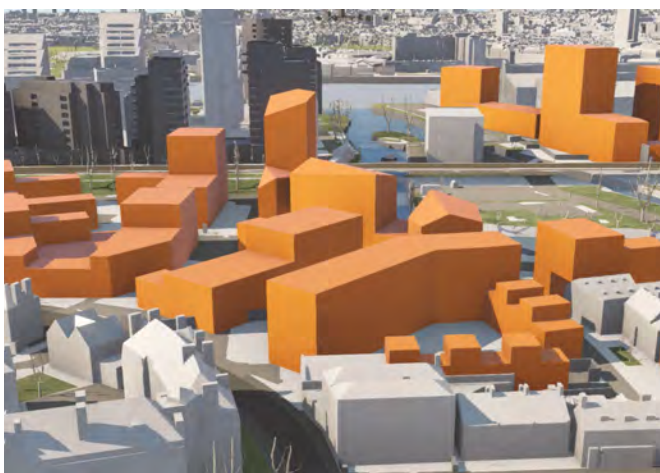
Fig. 384: View of the section of the Wandle Delta masterplan to the west of Bell Lane Creek. The blocks preserve the height of the old town and frontage along Armoury Way, while stepping up to provide height close to the railway line and the river.
